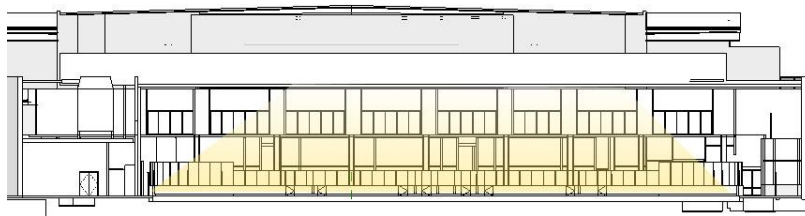
Figure 16. Community Rink Section (Daylighting)
